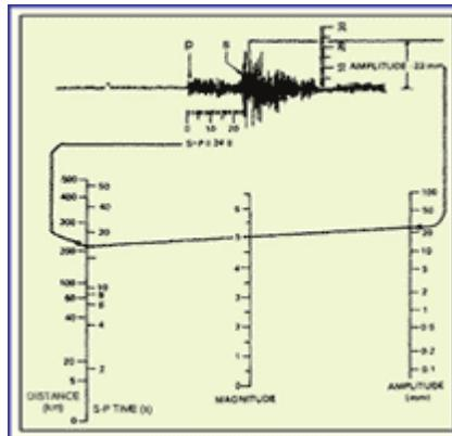
**Answer:** The local magnitude is defined as the logarithm of the maximum amplitude measured in microns on a seismogram written by Wood-Anderson seismograph with free period of 0.8 second, magnification of 2,800, damping factor of 0.8 calculated to be at a distance of 100 kms. The relative size of events is calculated by comparison to a reference event of  $M_L=0$ , using the formula,  $M_L = \log A - \log A_0$
